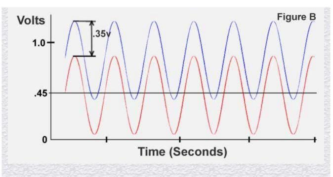
Almost all EFIE designs that are in use today work like the above graph, by adding a voltage to the output of the oxygen sensor. While this approach does work, and has been the only solution available for many years, it has 2 problems that make it not the ideal design.
